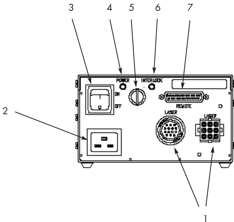
Figure 3.2 Front Panel Controls, Indicators and Connectors on the Laser Drive 9470 Power Supply
